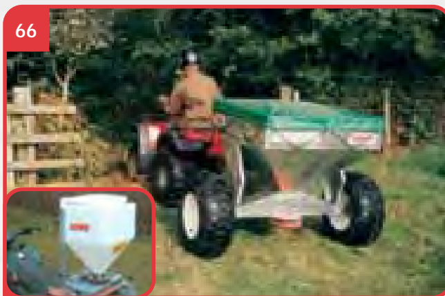
66 LGF TRAILED GAME FEEDER Suitable for larger game feeding requirements. Capacity is approx 320kg or approx 500kg with extension hopper. Handles flowable feeds, grain, pellets etc. Adjustable feed rate and geared, 12volt motor driven disc spreads up to approx 3m. Inset shows EBC-BD12 with 85ltr hopper and 12v belt driven motor to spread up to approximately 4m.
