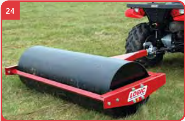
BR150 BALLAST ROLLER 1.5m. Liquid weight can be added to a maximum gross weight of approx 600kg, adjustable to suit ground conditions. Features include large 560mm dia heavy wall section drum for easy towing, 50mm dia axle, long life sealed bearings and adjustable rear scraper.
