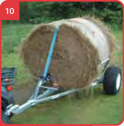
10 LBT TIPPING BALE TRAILER designed to self-load, carry and tip hay and straw round bales. Ideal for equestrian units and livestock farms, maximum load 600kg.
