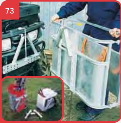
73 S300 'A' FRAME the basis of the System 30 can be supplied as a kit or as part of this S310KC Calf Crate product. The adjustable frame and installation kit ensure correct mounting. A ¼ turn spring catch releases equipment to be lifted off.
