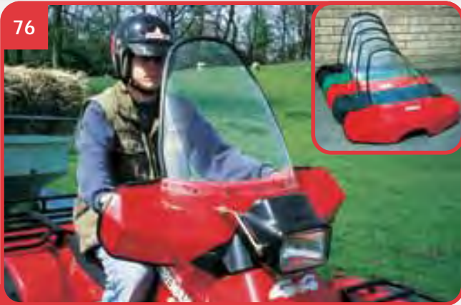
76 ATV WINDSCREENS have been specially designed for ATVs incorporating a stylish glass fibre handlebar fairing which creates an effective brush guard and protection from wind chill. Colour choice allows matching to specific ATVs. Screens are durable perspex with edge trim for added safety.
