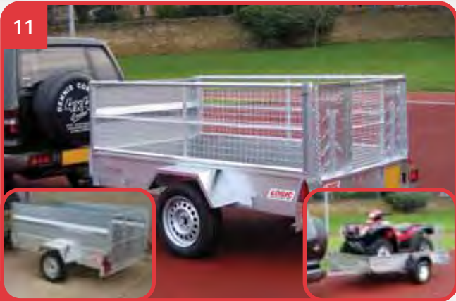
11 XT Range 2250 x 1310 x 300mm road legal trailers to suit a wide range of applications. Featuring maximum strength and durability with minimum unladen weight. Ideal for transporting an ATV and then used behind ATV off road. Main photo shows XT740 trailer fitted with solid headboard, mesh high sides and Logic style loading ramp tailgate. Inset left shows solid side option. Inset right shows XT610E fitted with XT106 ramp tailgate.
