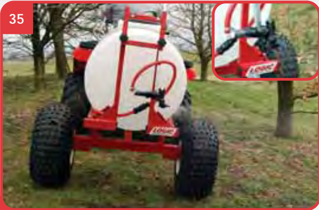
35 OBS107 boom fitted to TS400S trailed sprayer (also see picture 51) This nozzle can spray one side up to 3.5m and is ideal for working between established or newly planted trees and spraying steep ground such as railway embankments. The nozzle provides an accurate and even coverage over the ground but has the flexibility of not having to have a fixed boom. Inset shows a close up of the Nozzle. A Minimum of 9 ltr/min pump is required to run this nozzle.
