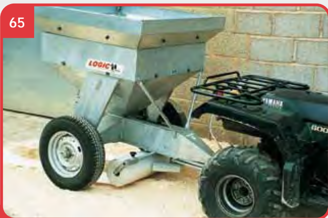
65 LCF160 CHICK FEEDER mechanises the time consuming job of laying feed onto paper in poultry houses. Features include hopper capacity up to 500kg, adjustable paper holder up to 1000mm width and 12 volt electrical remote on/off control allowing use with various vehicles, eg. Bobcat. One person can prepare a shed with 1500kg of feed in approximately 20 minutes.
