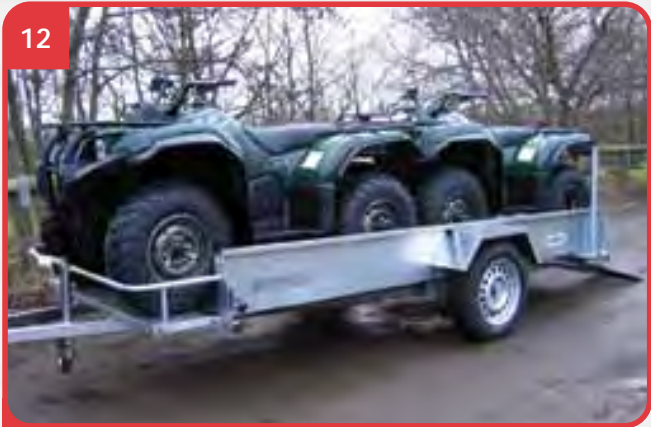
12 SXT Range 2995 x 1310 x 300mm road legal trailer, similar to XT range but with a drop down headboard and optional front bar which gives it a total body length up to 3500mm. Ideal for carrying a 6 wheeled ATV, Garden Tractors or 2 smaller ATVs such as sports or childrens models.
