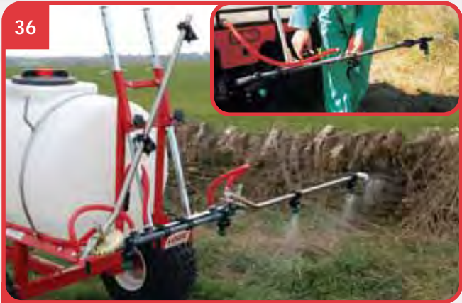
36 OBS BOOMS range from 1.5m (3 nozzle) to 3.5m (7 nozzle). The 3m and 3.5m booms are double folding with 2 breakback clutches. The main photo shows a OBS104 3m boom being used with only the 2 end nozzles and hedgerow nozzle being used to spray a field margin. All booms come with a hedgerow nozzle fitted to one side. Inset shows 1.5m boom which is rigid with single central breakback clutch.
